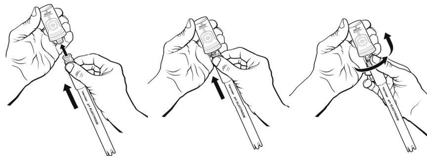
To prepare the electrode to make pH measurements, remove the storage bottle from the electrode by first unscrewing the lid and then removing the bottle and lid. Thoroughly rinse the lower section of the probe, especially around the bulb-shaped tip, using distilled or deionized water. **Note:** Do not completely submerge the sensor. The handle is not waterproof.
