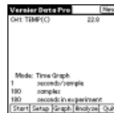
Data Pro will automatically identify auto-ID sensors, display the channel each is connected to, and display the current reading. Only active channels will be displayed. Tap **New** to detect the new sensors plugged into the LabPro. Older sensors that do not have auto-ID need to be set up manually.
